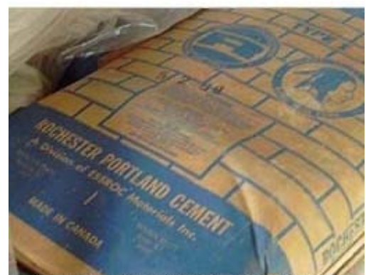
A sack of Portland cement will yield about 1.18 cu. ft. of cement
